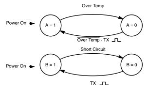
Note: Over Temp is an internal condition, not meant to be a logic signal.
